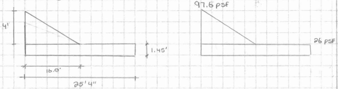
Snow drift on interior walls of fake Mansard Roof
